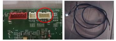
Solution: Check the connecter of sensor and slot, if loose or not plugged in, please connect again.
