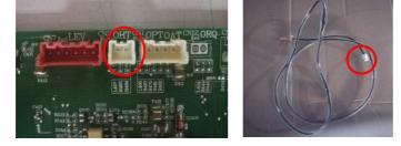
Solution: Check the connecter of sensor and slot, if loose or not plugged in, please connect again.
